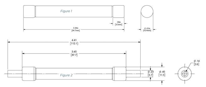
CC terminal (Fig. 2): Recommended crimping tool: T & B Sta-Kon ERG4002 #10 -12 AWG (6-4 mm<sup>2</sup>)
